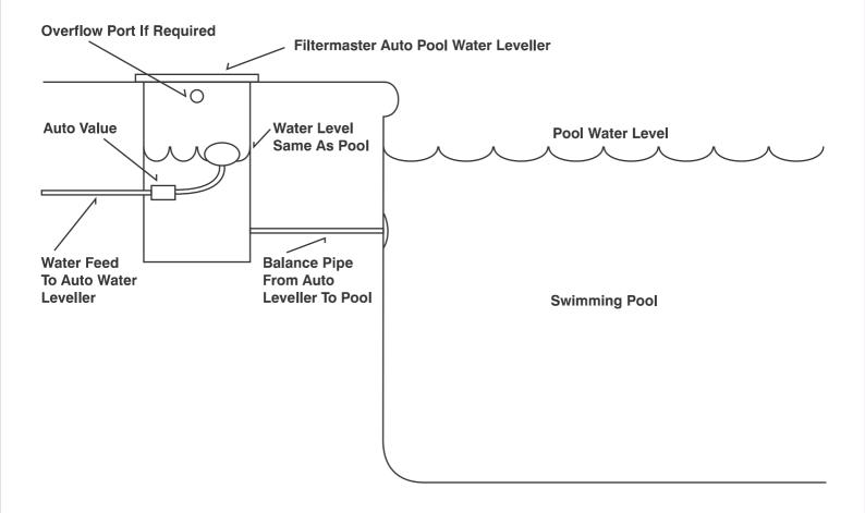
The Filtermaster Auto Pool Water Leveller is an accurate and reliable way to maintain a constant water level in your pool.
